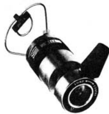
Figure 13.6 (a) Diagram of operation and (b) photo of two-position rotary injection valve. (Katz et al., used with permission.)
