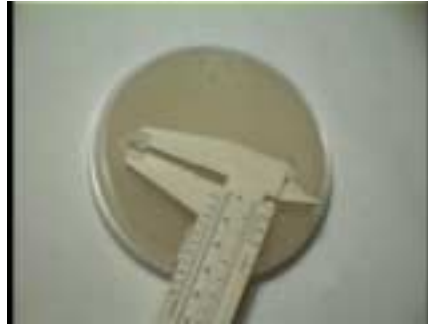
Figure 1. Calipers were used to measure the inhibition zones that resulted after the 24 hour incubation period[nicely done with the picture!]
